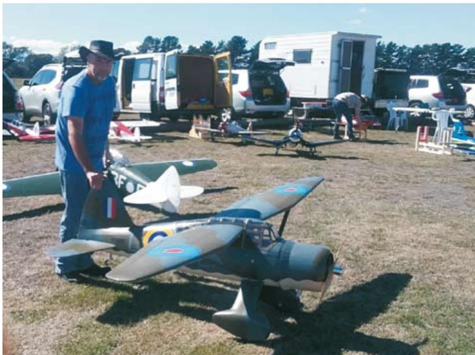
**Michael wheels out the Lysander. 118 inch wingspan, Powered by 50 cc PTE Engine with 22 x 8 prop, 9.6 kg**
