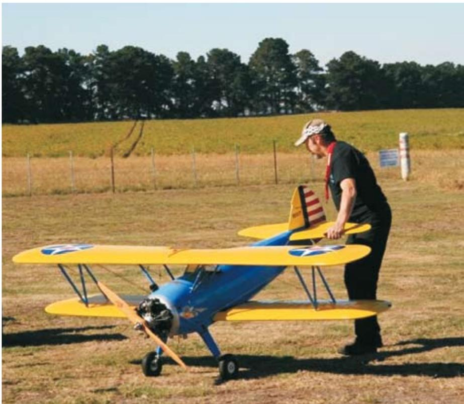
**Kevin Hay PT 17 1/3 scale Stearman, Wingspan 109 inch flying weight 24.8 kg, Engine Moki 215cc 5 Cylinder Radial**
